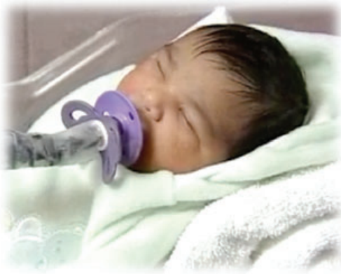
Figure 2. The photo shows a newborn sucking on the pacifier that is connected to a pressure transducer for measurement and stimulus control in the HAS procedure.
